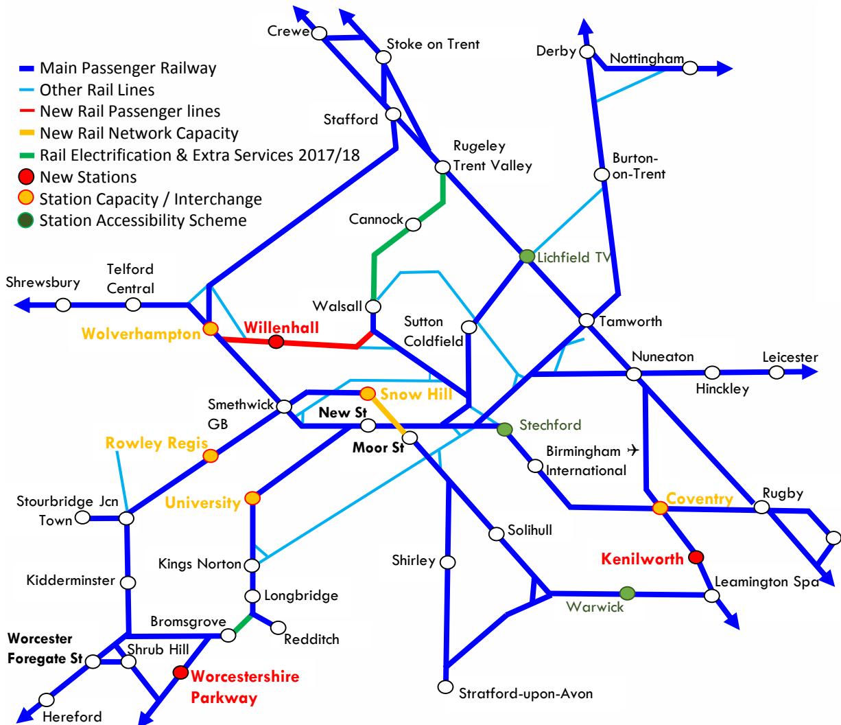
FIGURE 1 RAIL DEVELOPMENT PRIORITIES 2016 – 21: LONGER TRAINS, STATION CAPACITY
